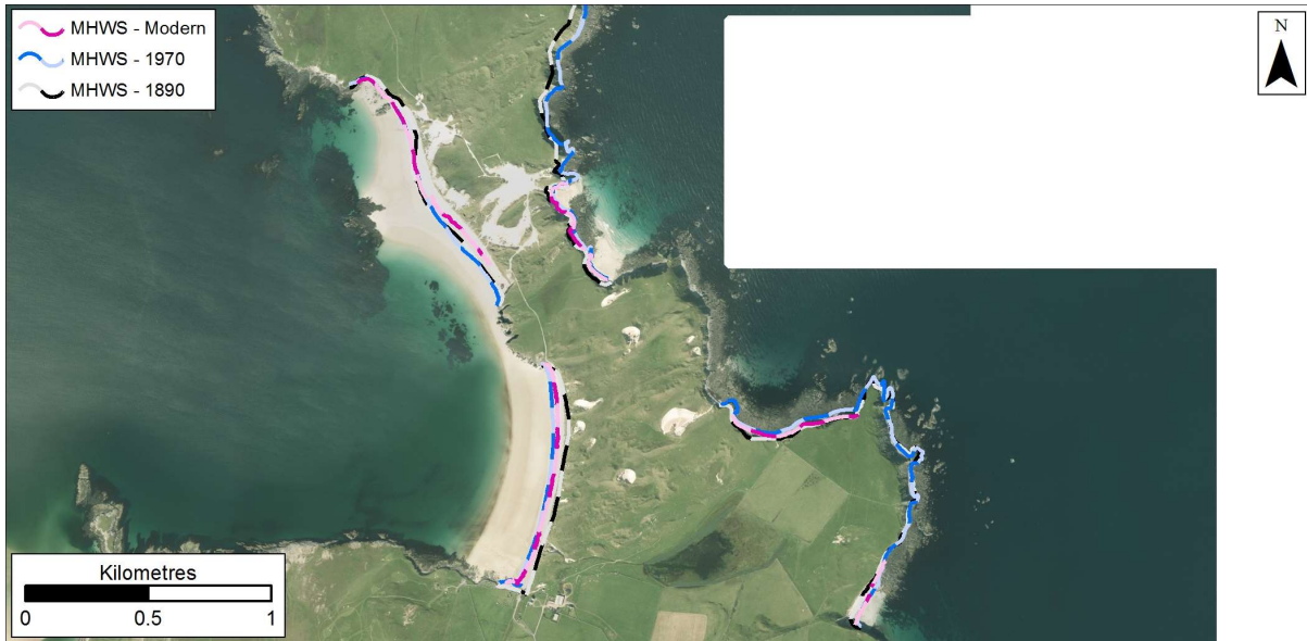
Figure 4.10: MHWs position in 1890, 1970s, and Modern datasets at Balnakeil. Getmapping are our current providers of Scotland-wide digital aerial imagery© Getmapping plc.
