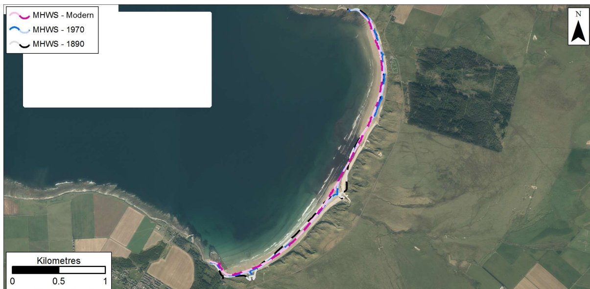
Figure 4.3: MHWs position in 1890, 1970s, and Modern datasets at Dunnet Sands. Getmapping are our current providers of Scotland-wide digital aerial imagery© Getmapping plc.
