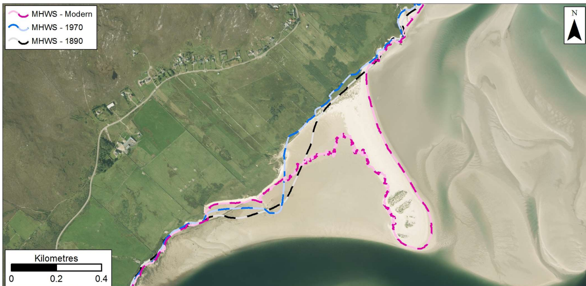
Figure 4.8: MHWS position in 1890, 1970s, and Modern datasets at the Kyle of Tongue. Getmapping are our current providers of Scotland-wide digital aerial imagery© Getmapping plc.
